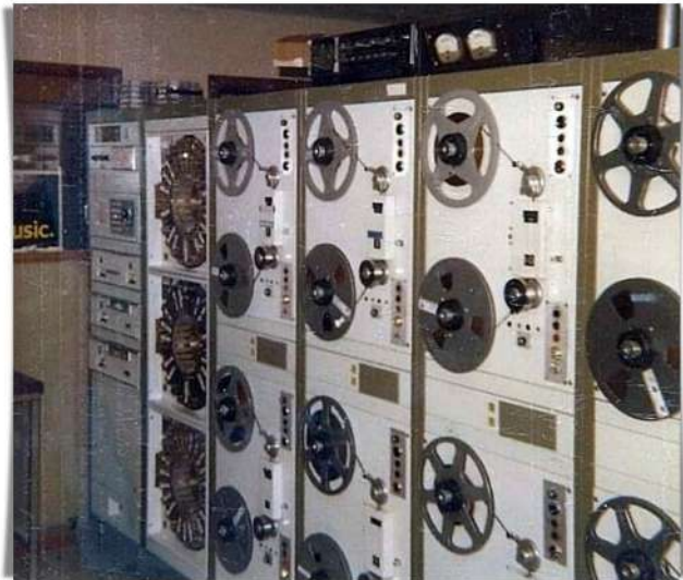
KGOR automation system of tape cartridge carousels and open-reel tape players at 5010 Underwood, co-located with KFAB 1110. (Courtesy: Norm Gruenke.)
